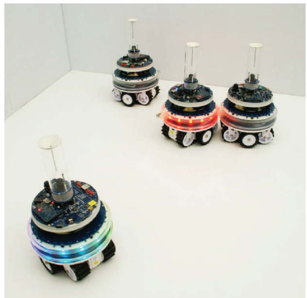
Figure 3. The foot-bot robotic platform. The foot-bot has a differential drive system that uses a combination of tracks and wheels to provide mobility on rough terrain. Two of the foot-bots in this figure have illuminated their LED communication ring. These red-green-blue (RGB) colored signals are detectable by the onboard cameras of other foot-bots.
